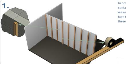
In order to prevent a sound bridge due to direct contact between the wood slats and the wall, we recommend applying our soni NBR sealing tape to both sides of the slats and then fixing these to the wall using dowels and screws.
